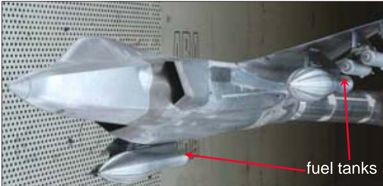
This wind tunnel model of F-35 features an optimized external fuel tank.
