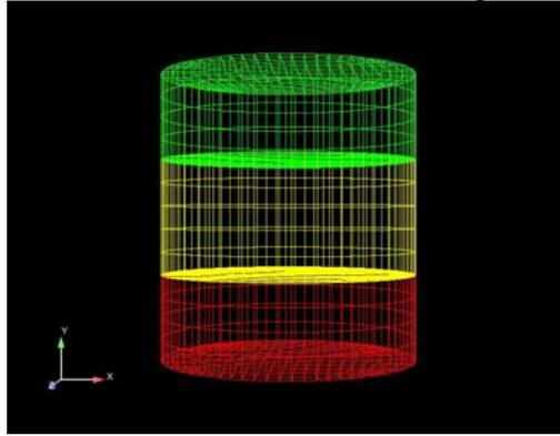
*Figure 4. 3 disc model with filled rubber as the middle disc (in yellow)*
