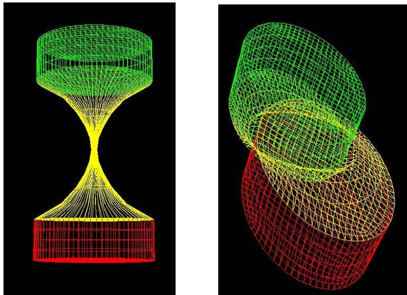
*Figure 5. Axial Mode (left) and Shear Mode (right) for 3-disc model*
