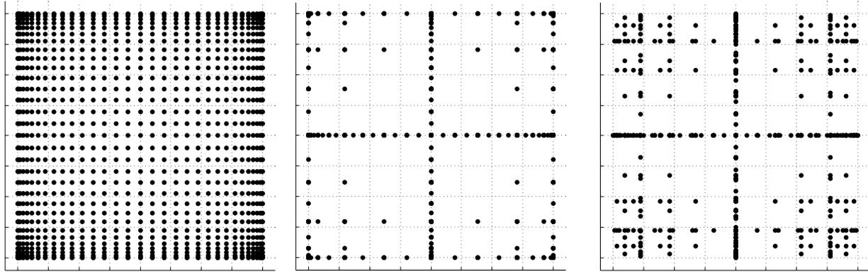
Figure 2. For a two-dimensional parameter space ( $n = 2$ ) and maximum level  $w = 5$ , we plot the full tensor product grid using the Clenshaw-Curtis abscissas (left) and isotropic Smolyak sparse grids  $\mathcal{A}(5, 2)$ , utilizing the Clenshaw-Curtis abscissas (middle) and the Gaussian abscissas (right).
