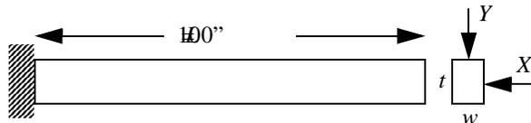
Figure 12. Cantilever beam test problem.
