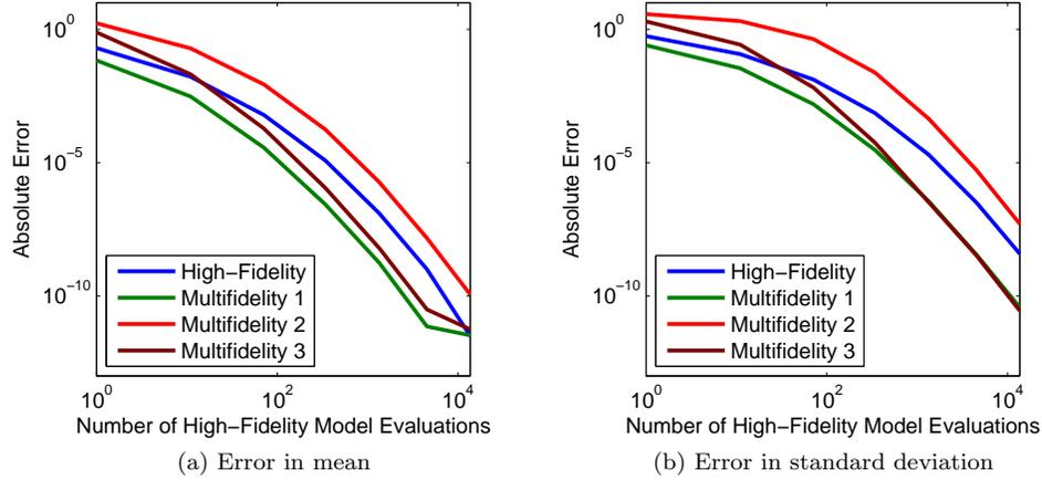
Figure 3: Convergence of single-fidelity PCE and multifidelity PCE with additive correction using isotropic sparse grids for the short column example. The multifidelity sparse grid level offset is set to one.
