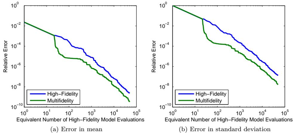
Figure 6: Convergence of single-fidelity PCE and multifidelity PCE with additive correction using adaptive generalized sparse grids for the elliptic PDE example.
