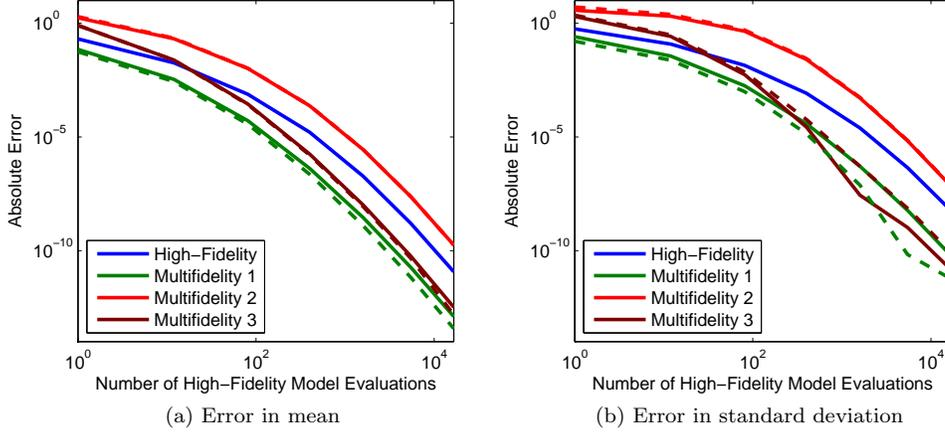
Figure 5: Convergence of single-fidelity PCE and multifidelity PCE with additive correction using isotropic sparse grids for the short column example. The multifidelity sparse grid level offset is compared using  $r = 1$  from Figure 3 (solid lines) and  $r = 2$  (dashed lines).
