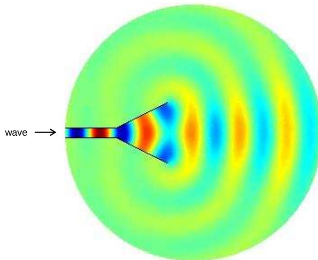
Figure 7: 2-D horn geometry and the propagation of acoustic waves.
