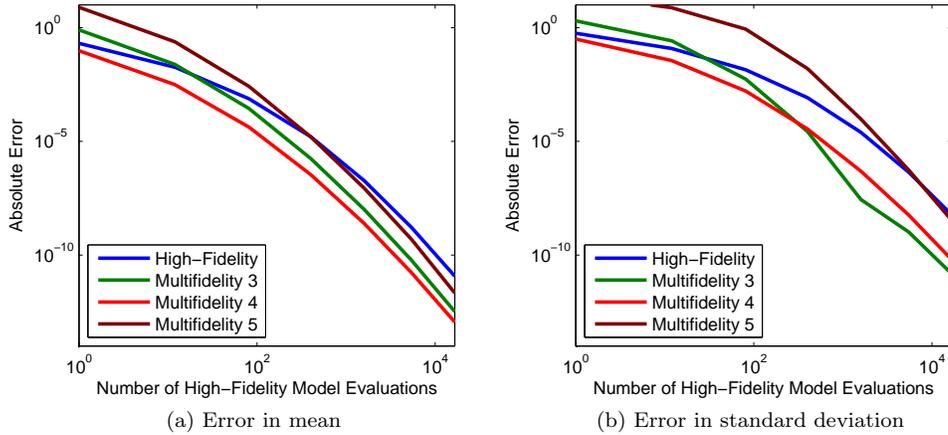
Figure 4: Convergence of single-fidelity PCE and multifidelity PCE with additive correction using isotropic sparse grids for the short column example. The multifidelity sparse grid level offset is set to one.
