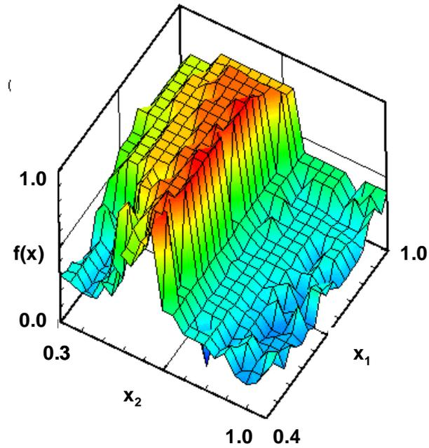
Figure 1. Parameter study data from Giunta (2002a), showing a steep-walled cliff adjacent to the maximum values (dark/red region) of the objective function,  $f(x_1, x_2)$ . The global maxima are not robust to perturbations in  $x_2$ .
