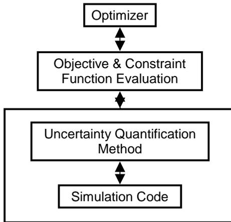
Figure 3. A notional optimization under uncertainty problem formulation, with an uncertainty quantification (UQ) method embedded inside an optimization loop.
