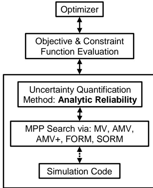
Figure 6. Optimization under uncertainty with an analytic reliability method for uncertainty quantification.
