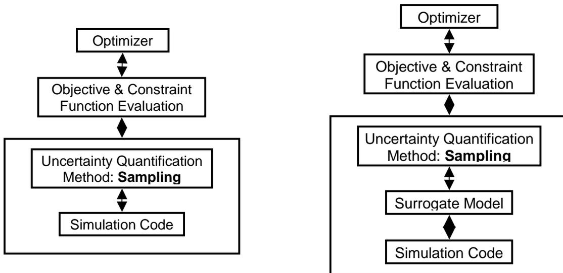
Figure 4. Optimization under uncertainty with a sampling-based method for uncertainty quantification.
