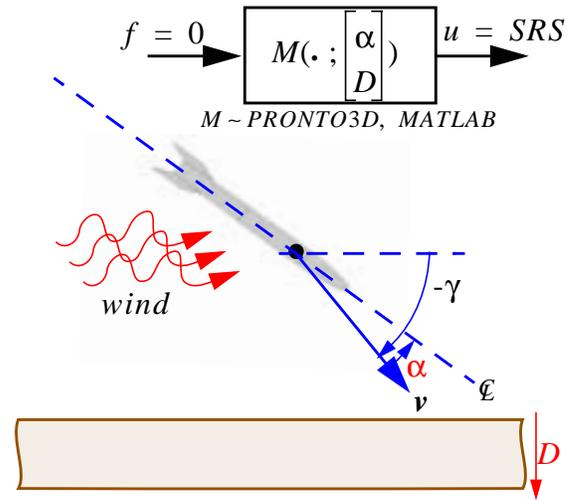
Figure 6. Schematic of the penetration system.
